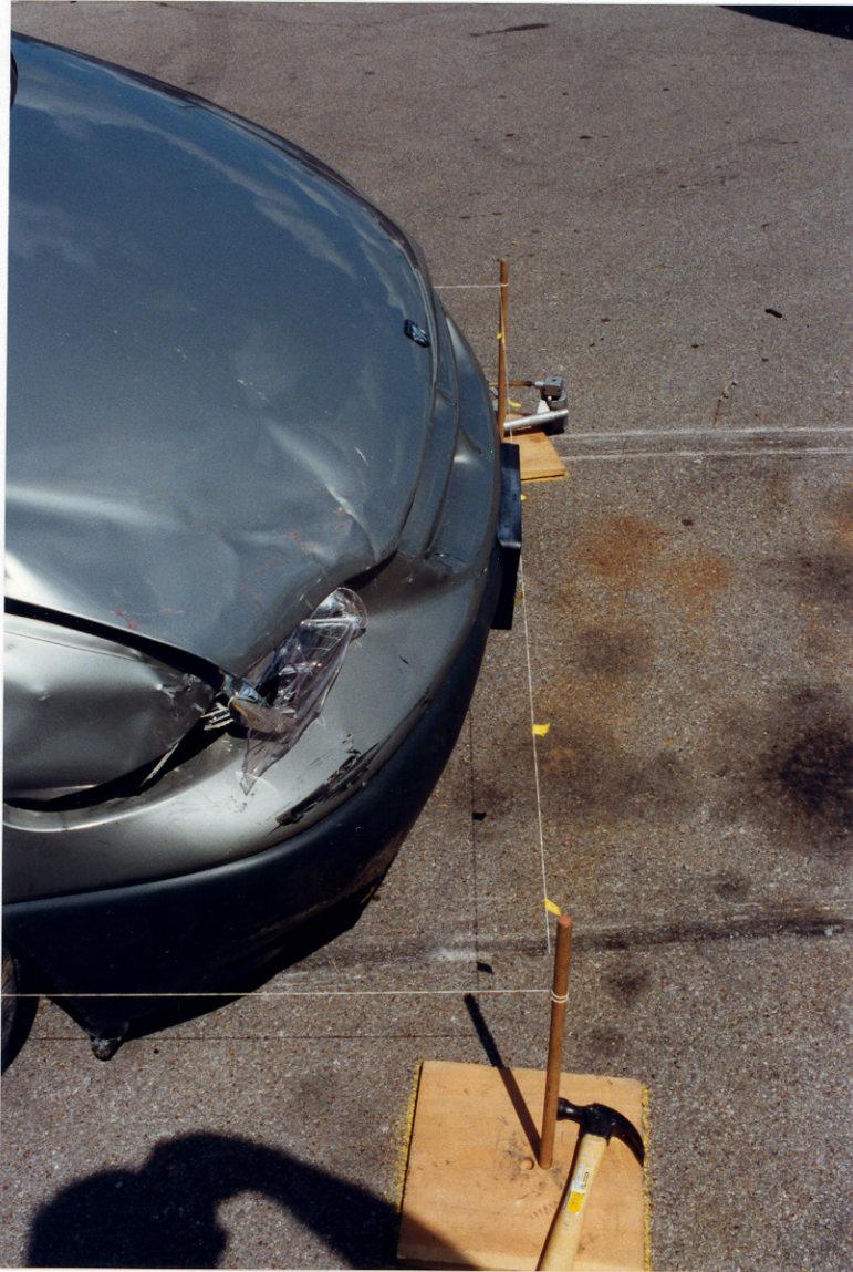
47. Right lateral view of the damage to the front of the Dodge Caravan.
